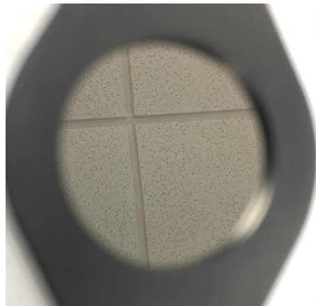
Figure 4.3: Image showing the mount and mirror used to generate BRDF data. The sample is a coated aluminum that is highly specular, as evidenced by the reflection of the ceiling tiles on the mirror. The sample appears quite smooth with no visible scratches or machine lines.
